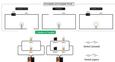
Switches can be placed in a parallel circuit, so that 1 light can be turned on while another is off (just like in a house).
